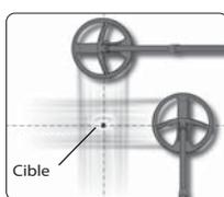
If you are having difficulty locating the target then sweep the place where you heard the sound. Move a quarter turn around the spot and begin sweeping again in the same way. You should then locate the precise zone containing your target at the intersection of the two sweeps where the sound is loudest.
