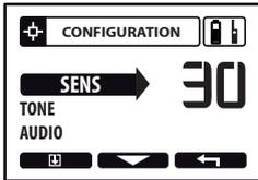
The MI-6 has 50 levels of sensitivity via the remote control.
