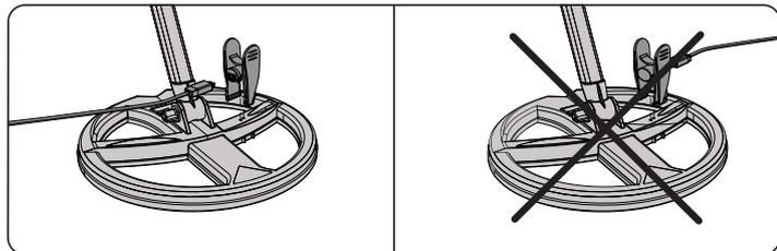
Ensure that the clamp is the right way round before connecting it to the coil. Do not adjust after fitting, it can take up to 10 seconds for the led to activate.
