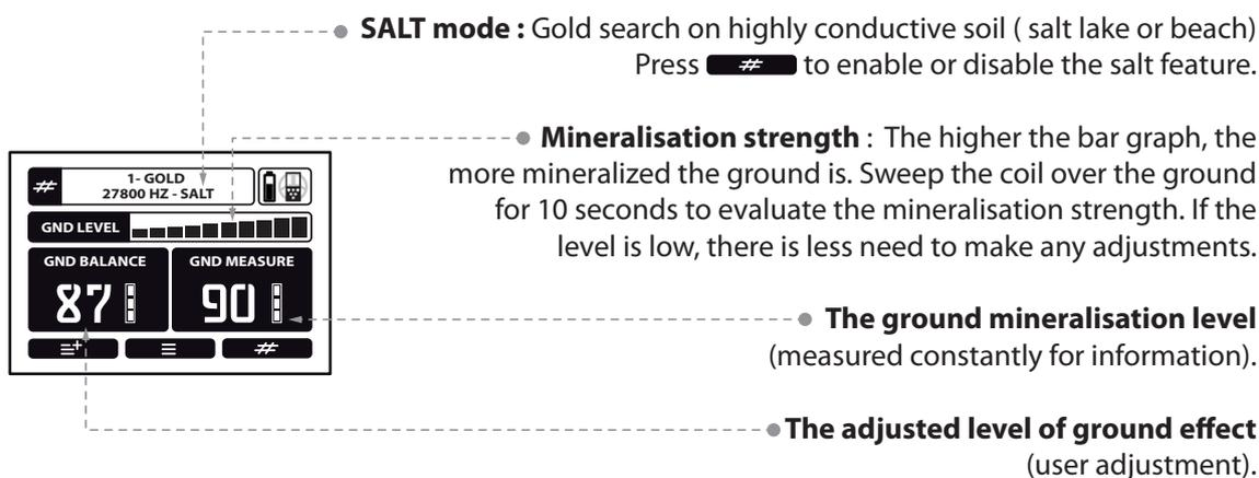
The diagram shows a detector's ground balance screen with the following elements:
