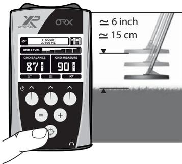
On the controller, press the “Ground Balance” button
