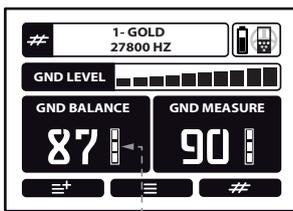
You can manually adjust the ground rejection levels.
