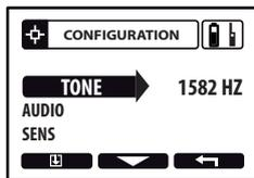
The MI-6 audio PULSE tone can be adjusted from the remote control, tones range from 120 to 1582 Hz. (Audio PULSE mode only).
