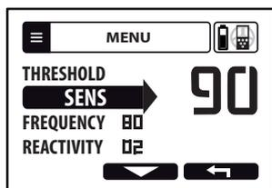
1 Adjust the Sensitivity level (from 0 to 99) with
