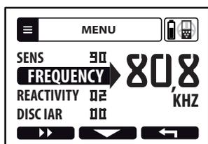
You can shift your operating frequency slightly to avoid interference generated by another detector in close proximity or electromagnetic interference (EMI).
